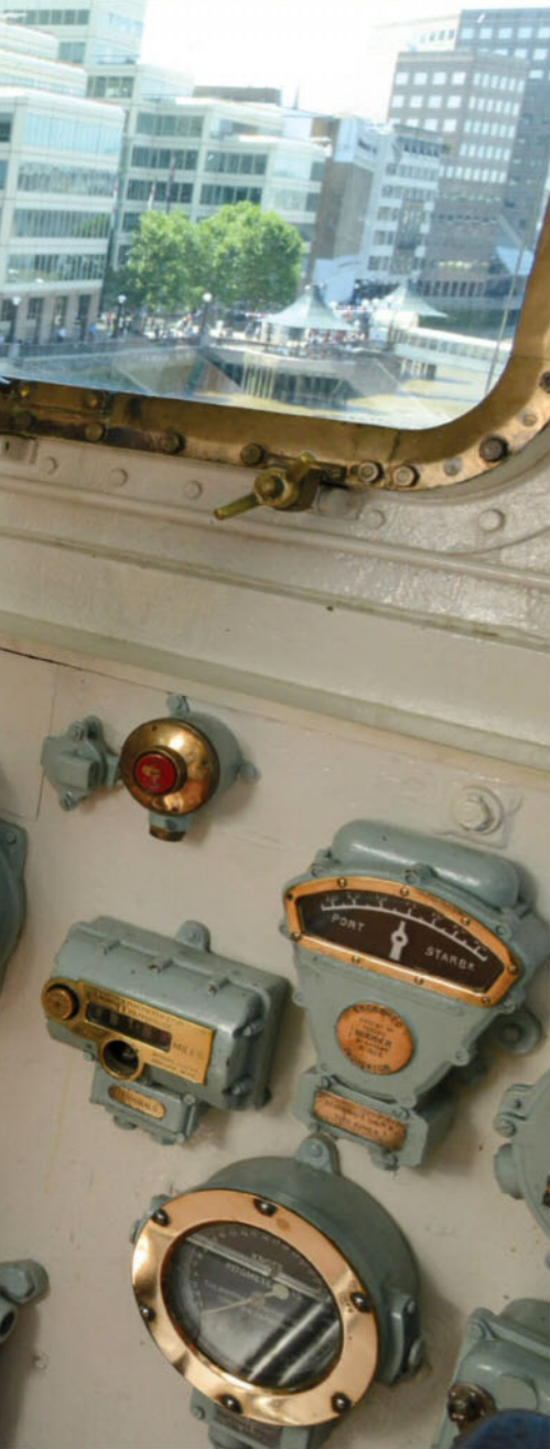
Belfast contains a World War II computer (centre) that calculated the firing angles for the guns. Remarkably, the technology for these machines actually dates back to World War I
